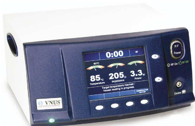
Figure 2 RF generator, version 2. Note clear displays of time, temperature, impedance, and watts. (Courtesy VNUS Medical Technologies, San Jose, CA).
